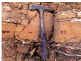
A layer of rocks with 30 cm thickness containing a percentage of (2% of P_2O_5 )- Jebel Abyad W.Dongola - N.Sudan
