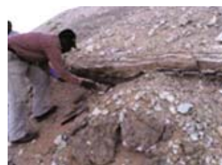
A layer of rocks with 30 cm thickness containing a percentage of (7% of P_2O_5 )- Jebel Abyad W.Dongola - N.Sudan
